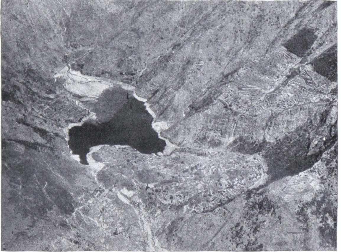
2. "Natural erosion" occurs throughout the Himalayas. This small lake, in Jajarkot District, W. Nepal, was formed by a landslide that blocked a small stream. The landslide left the scar on the hillside, right, and now forms the foundation for a small village and cultivations.
